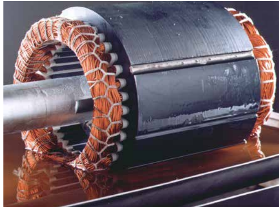
An impregnation resin applied by roll through
